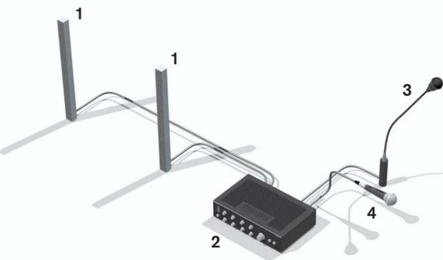
The XLA 3200 loudspeakers are connected to a Plena mixer amplifier (2). The loudspeakers are connected directly on the 100 V loudspeaker lines. One or two microphones (3+4) are connected to the Plena by means of a balanced line. If a condenser microphone is used, the length of this line is not critical.
