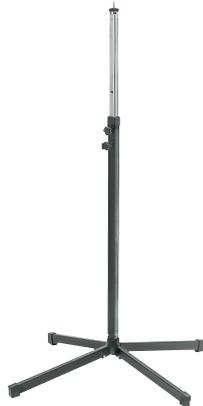
The robust LBC 1250/00 loudspeaker floor-stand is height-adjustable between 1.2 and 1.9 m, and has a wide leg-span to ensure stability. Finished in a tough matt black lacquer, the stand is collapsible, measuring just 1.5 m when folded. For compact storage or shipping, the folding legs can be unscrewed from the outer tube. A standard 1/2" Whitworth threaded stud with locking nut heads the adjustable nickel-plated inner tube.
